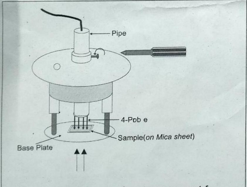
Fig. 3 shows four probe arrangement for mounting sample.
