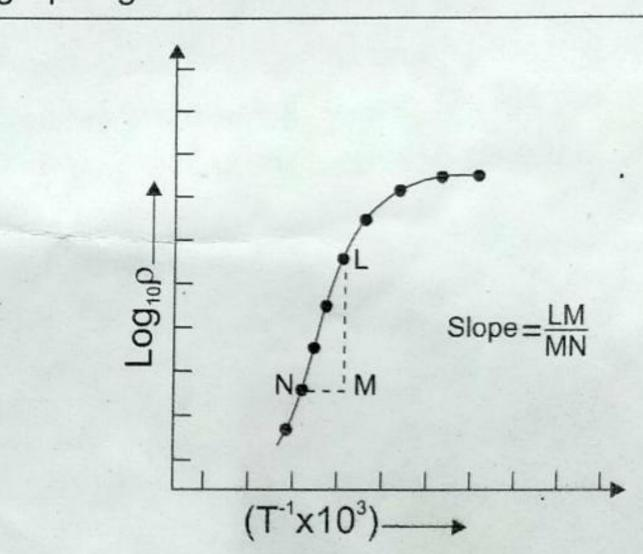
Fig.4 A typical graph showing the resistivity of Germanium crystal as a function of inverse temperature
