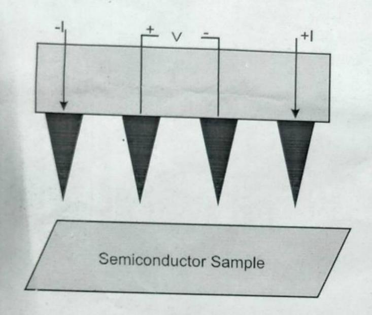
Fig. 1. Schematic diagram of 4-probe measurement.
